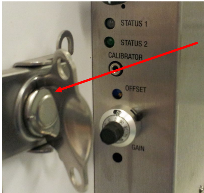
Figure 107 Circuit Offset Potentiometer Location
