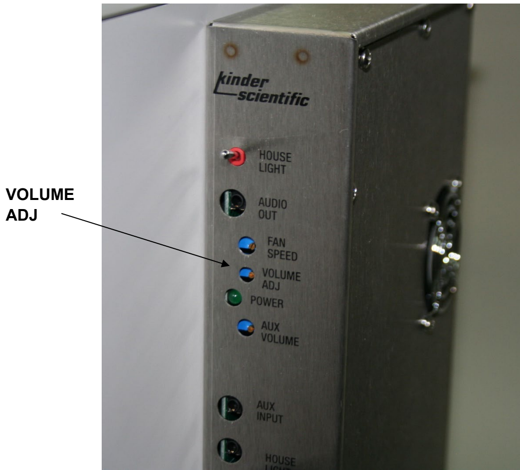
Figure 123 Volume ADJ Potentiometer Location
